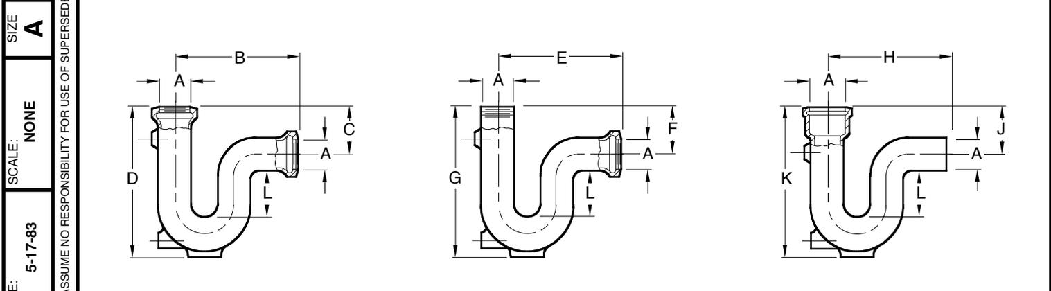
Fig. 7220T . . . FEMALE THREADED INLET AND OUTLET
