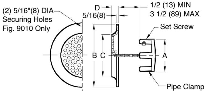
Fig. 9005 . . . WITH PIPE CLAMP
