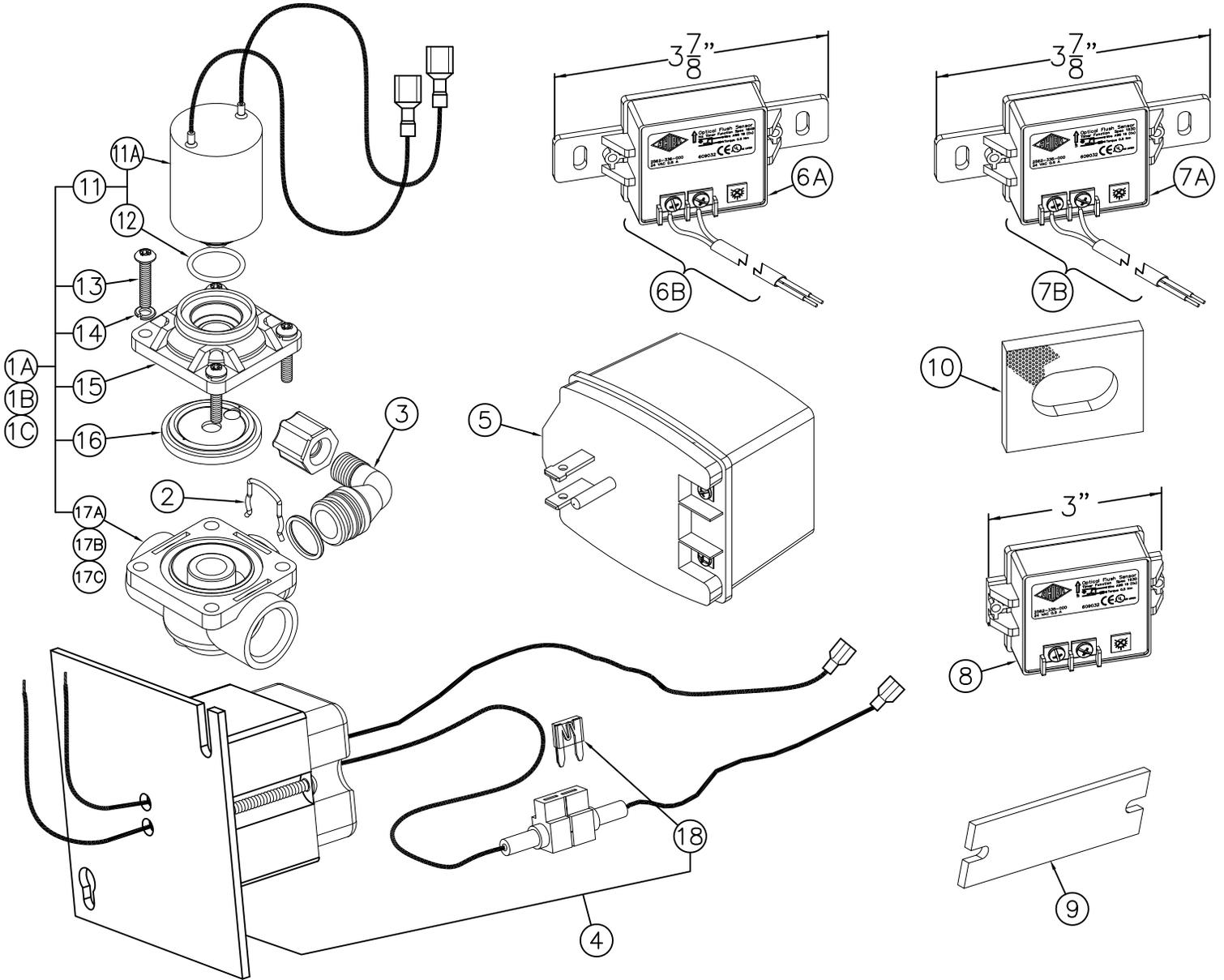
NOTE: WHEN REPLACING THE SENSOR ON CIRCULAR SPRAYHEADS ENSURE TO REPLACE THE SENSOR FOAM GASKET AS WELL.
