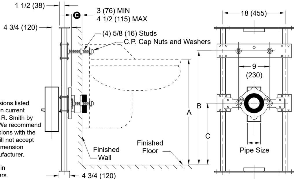
**NOTE:** The rough-in dimensions listed on this drawing are based on current information available to Jay R. Smith by the fixture manufacturers. We recommend that you verify these dimensions with the fixture manufacturer. We will not accept responsibility for rough-in dimension changes by the fixture manufacturer.
