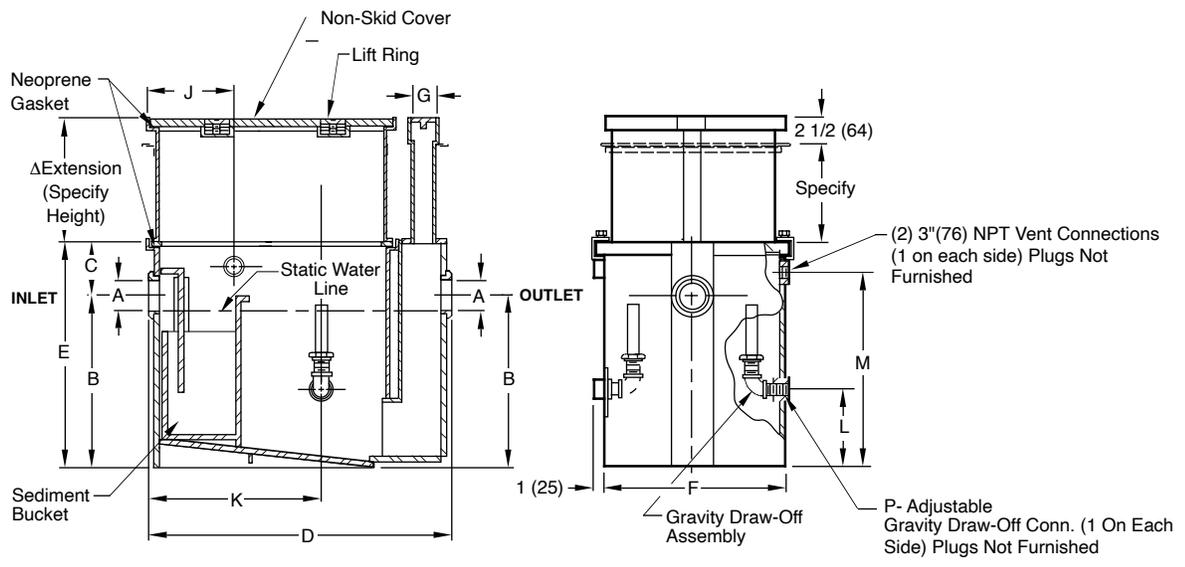
**NOTE:** Interceptor shall be vented on outlet side per local code requirements.
