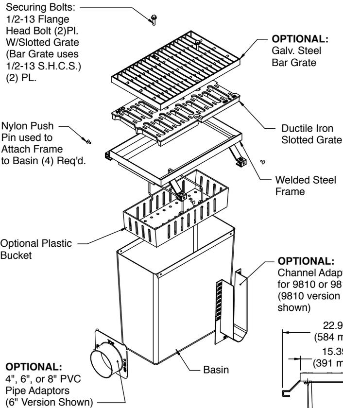
**EXPLODED ASSEMBLY DETAIL**
