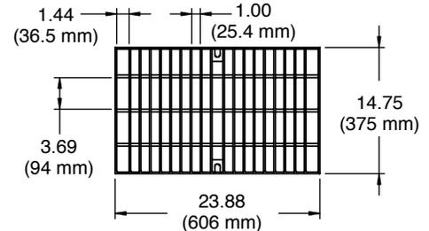
**Galvanized Steel Grate Detail**
