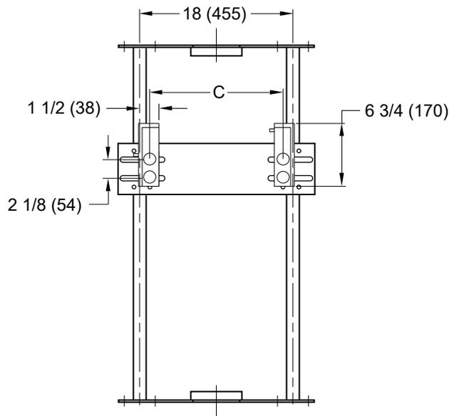
**Fig. 0761. . . . WITH ACID RESISTANT COATED EXPOSED ARMS FOR FLAT SLAB AND HIGH BACK LAVATORIES**
