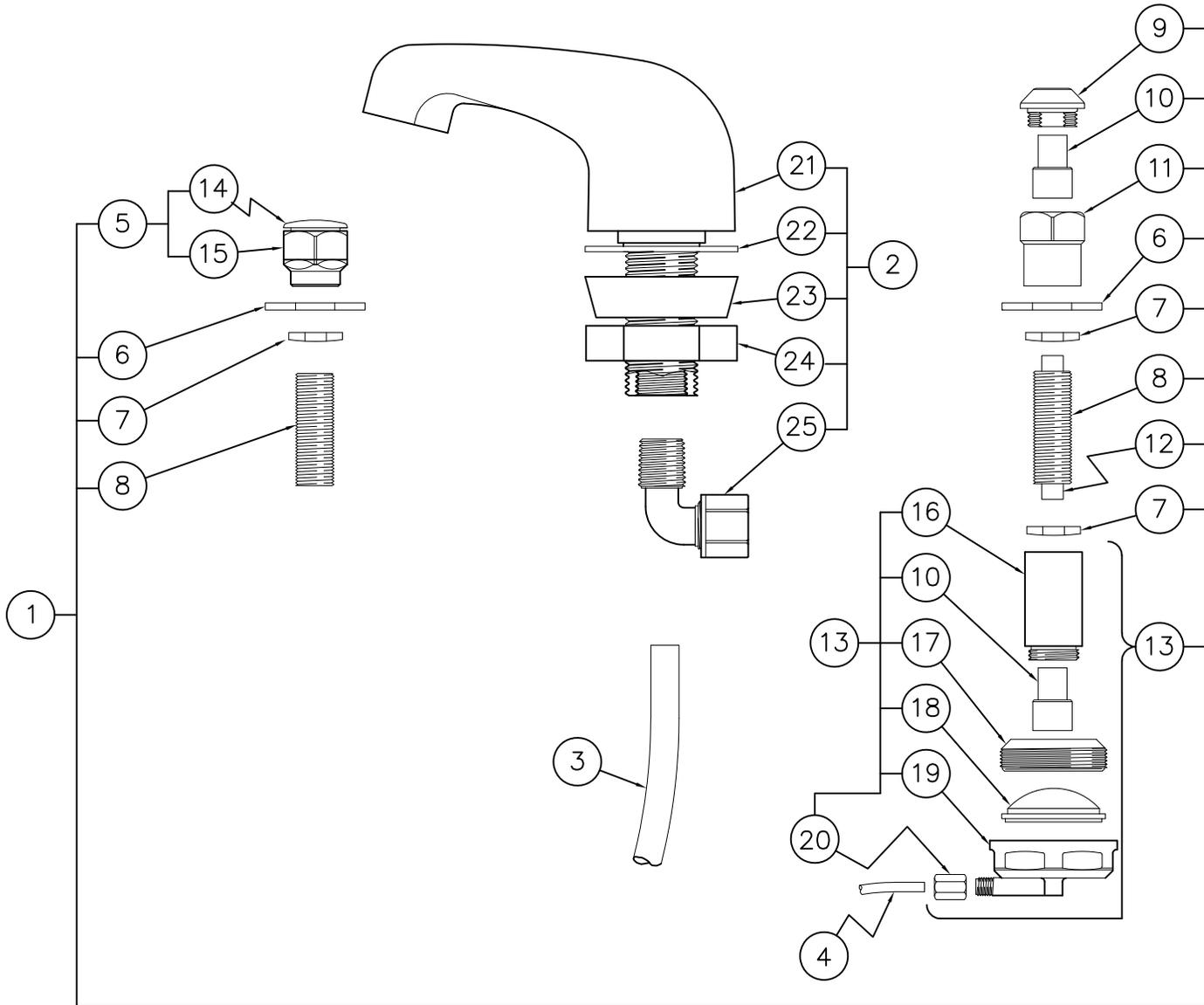
**PUSHROD ACTIVATED AIR-CONTROL PUSHBUTTON ASSEMBLY FOR 8" WALL**
