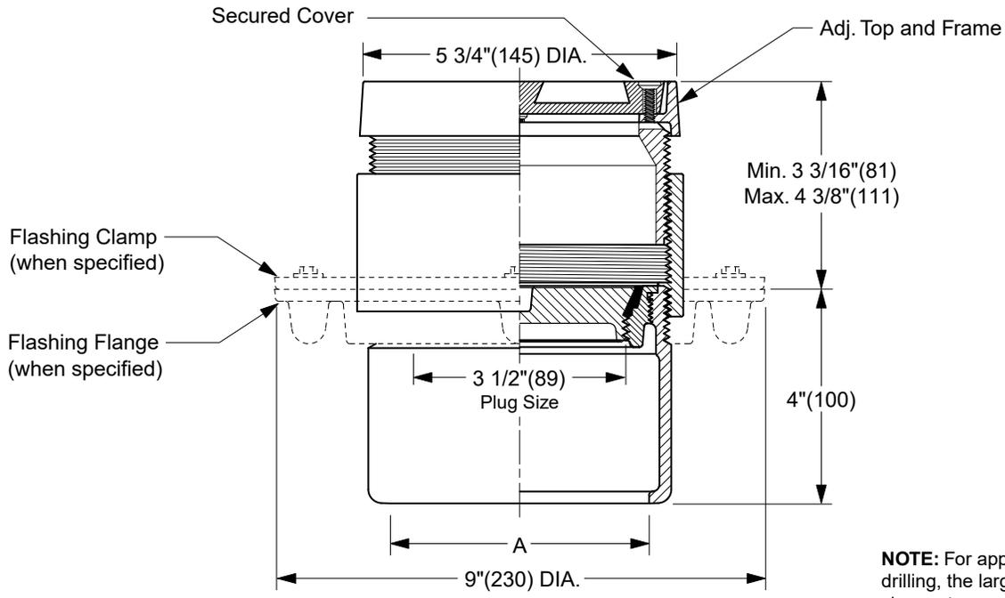
**NOTE:** For applications using core drilling, the largest diameter of the cleanout assembly is 6 5/16" (160).
