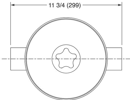
**NOTE:** Allow 9 (230) of clearance above interceptor for bucket removal.
