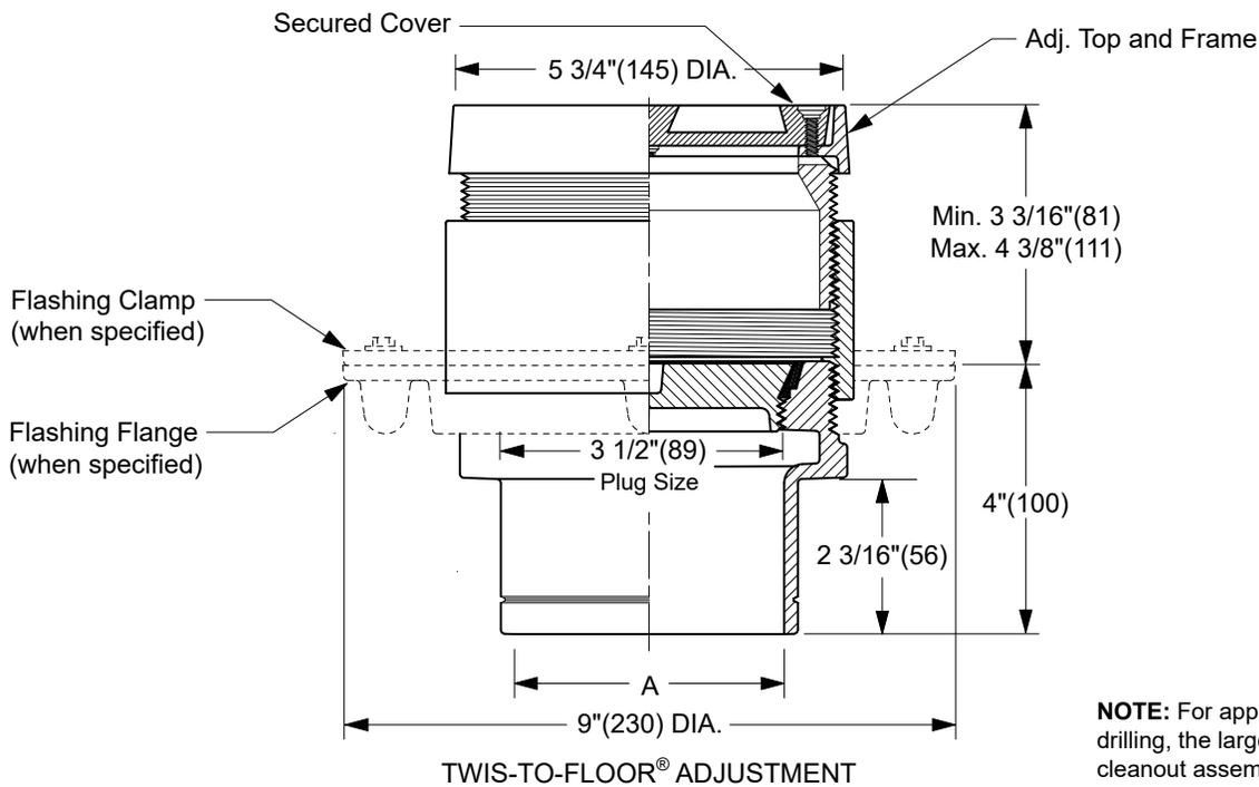
**NOTE:** For applications using core drilling, the largest diameter of the cleanout assembly is 6 5/16" (160).
