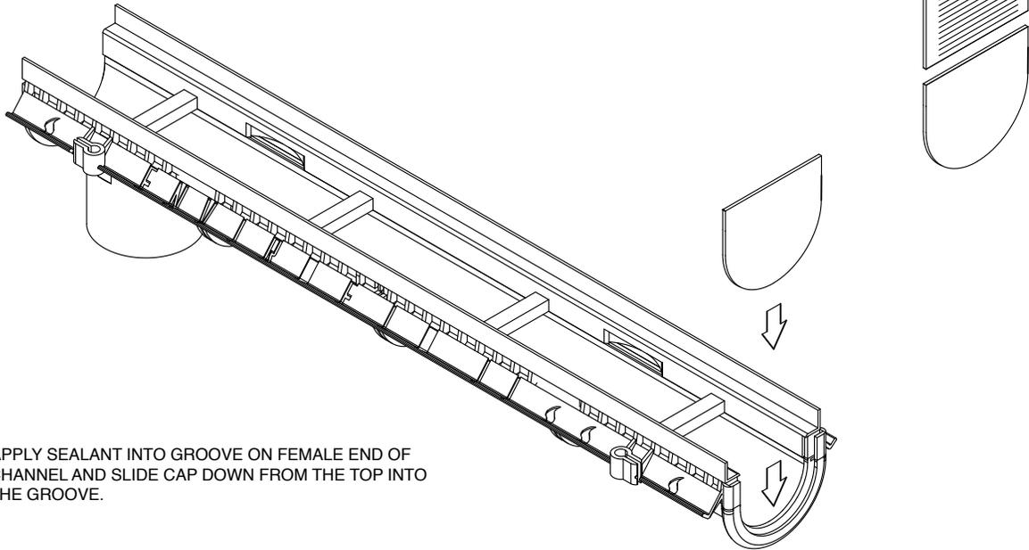
**STEP 2:** APPLY SEALANT INTO GROOVE ON FEMALE END OF CHANNEL AND SLIDE CAP DOWN FROM THE TOP INTO THE GROOVE.
