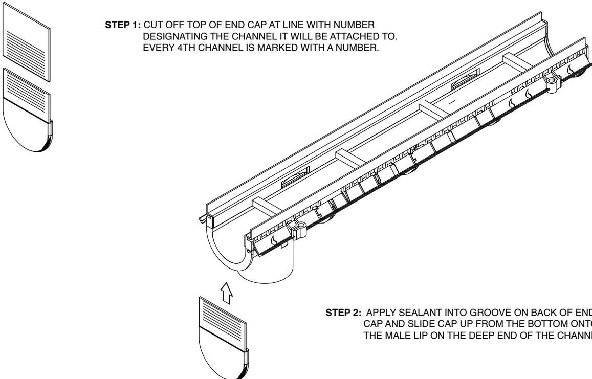
**STEP 2:** APPLY SEALANT INTO GROOVE ON BACK OF END CAP AND SLIDE CAP UP FROM THE BOTTOM ONTO THE MALE LIP ON THE DEEP END OF THE CHANNEL.
