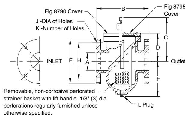
Fig. 8790. . . . WITH YOKE TYPE COVER
