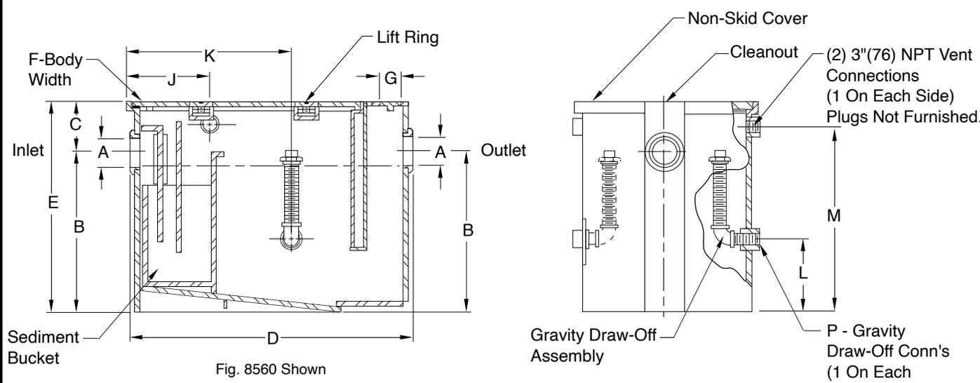
**NOTE:** Interceptor shall be vented on outlet side per local code requirements.
