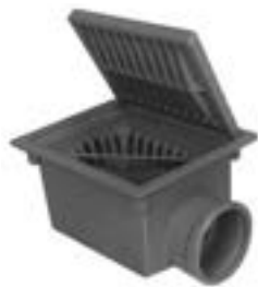
FIG. 2475 HEAVY DUTY TRAFFIC FLOOR DRAIN W/SIDE OUTLET, HINGED GRATE AND FREE STANDING SEDIMENT BUCKET
