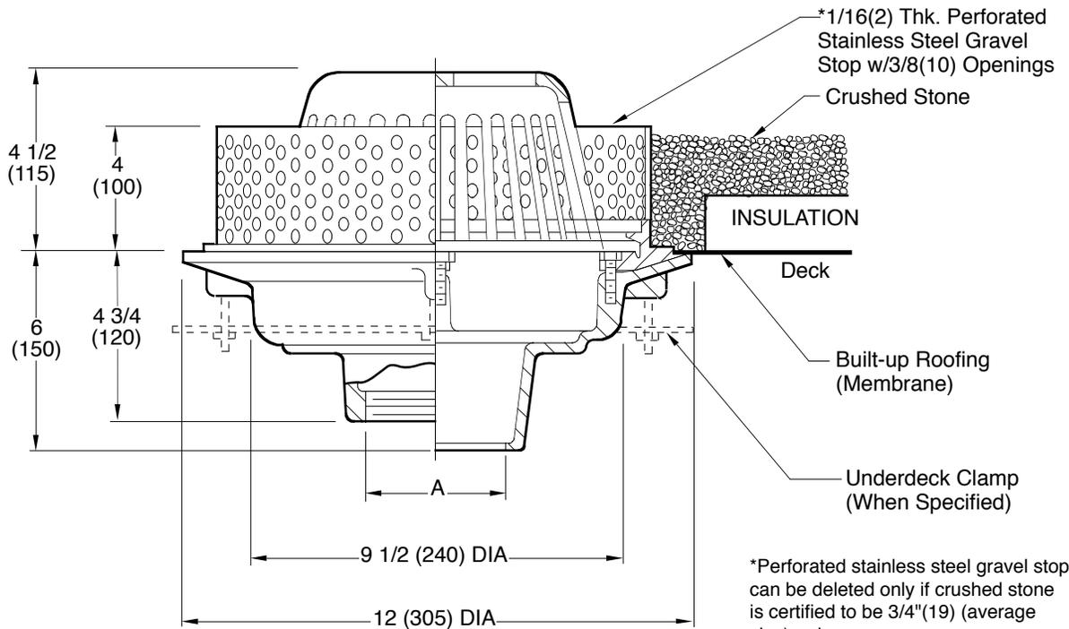
\*1/16(2) Thk. Perforated Stainless Steel Gravel Stop w/3/8(10) Openings
