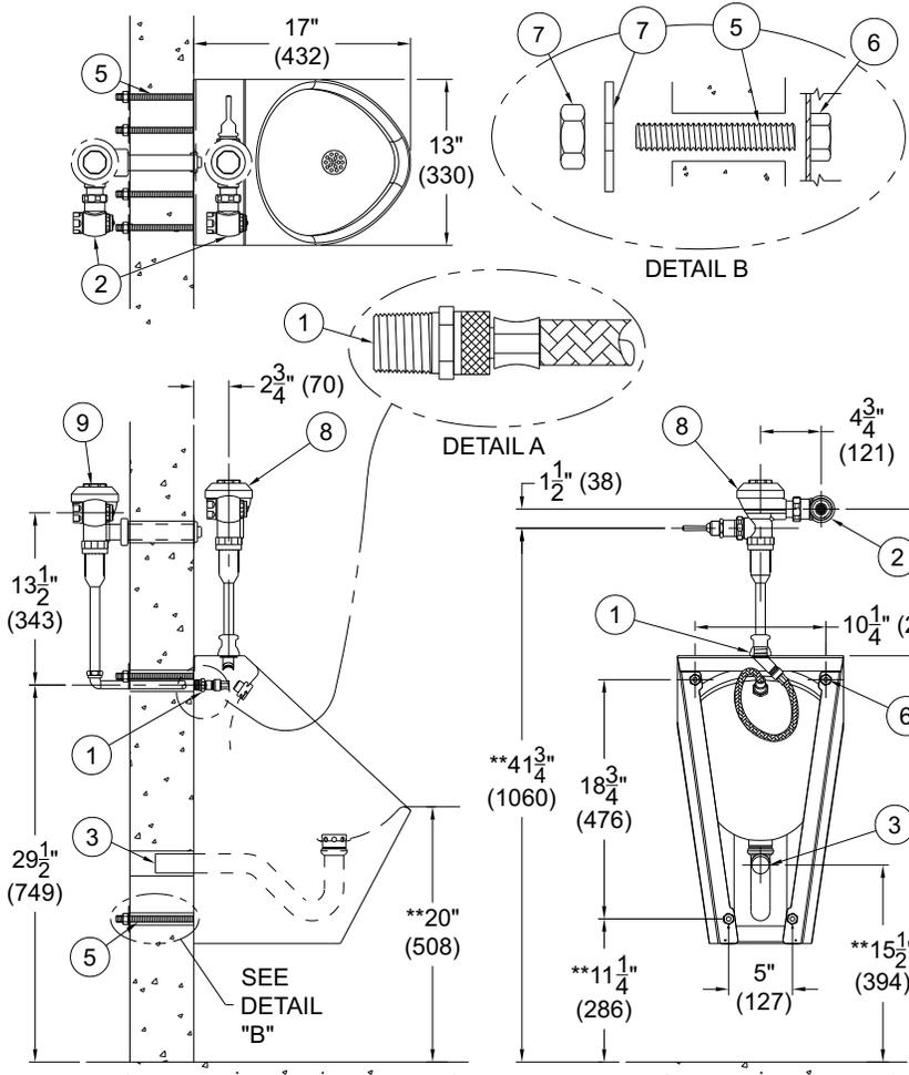
**NOTE: REFER TO ADA GUIDELINES FOR COMPLETE INSTALLATION REQUIREMENTS. ALL VERTICAL DIMENSIONS INDICATED (\*\*) DECREASE PROPORTIONALLY WITH ADA RIM HEIGHT:**
