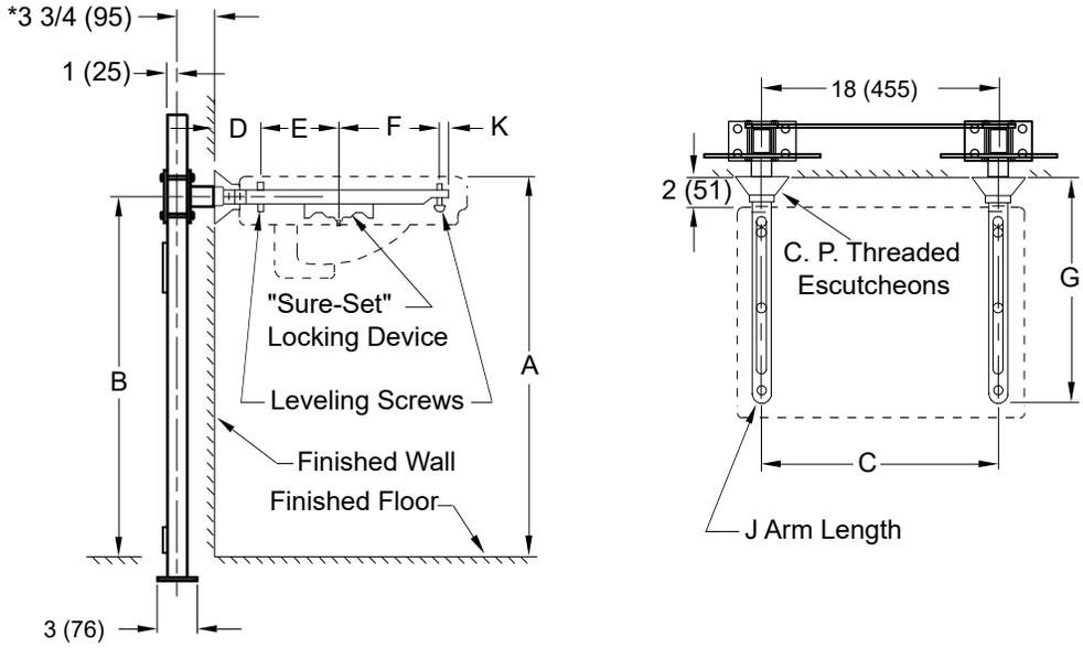
**Fig. 0710 (-E) . . . FOR FLAT SLAB LAVATORIES (shown)**
