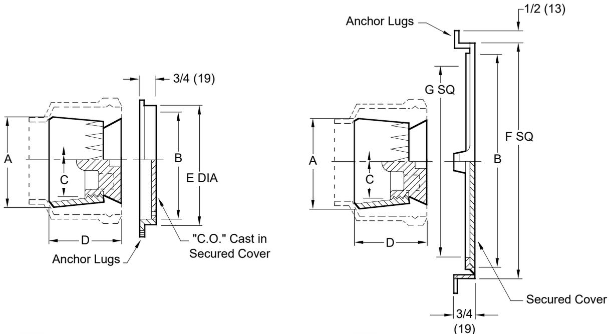
FIG. 4438C . . . . FLUSH-WITH-WALL COVER
