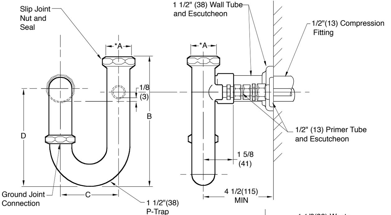
**IMPORTANT:** P-Trap must be mounted parallel with wall and outlet left of the lavatory drain.
