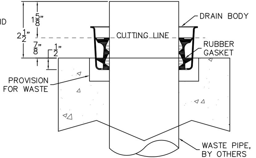
**WASTE PIPE CUTTING DETAIL**
