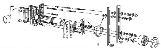
**-M40 WATER CLOSET SUPPORT FOR WIDE PIPE CHASE (USE WHEN Ⓢ DIMENSION EXCEEDS 7" (180))**
