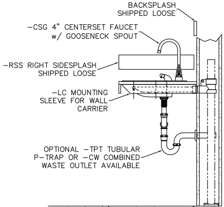
**MOUNT OPTIONAL -LC MOUNTING SLEEVE TO WALL CARRIER**
