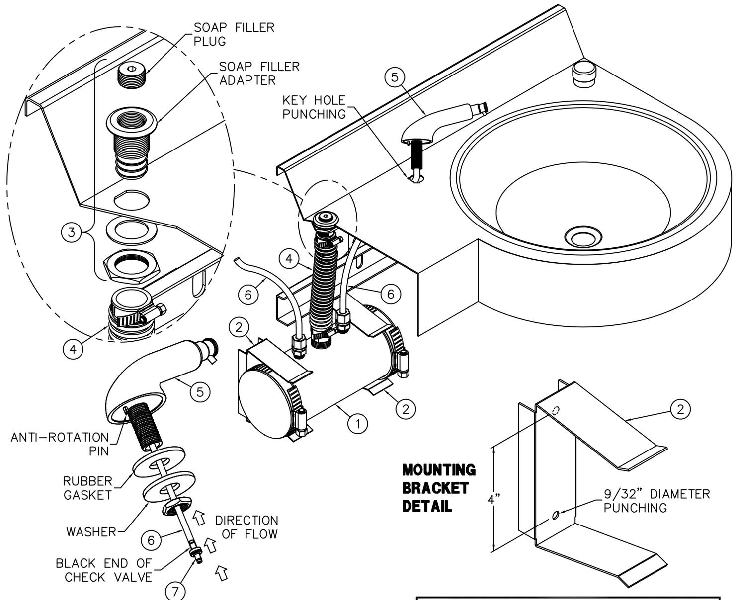
FOR BEST RESULTS INSTALL SOAP RESERVOIR FILL HOLE DIRECTLY BELOW SOAP FILLER ON DECK WITH REFILL TUBE AS SHORT AND STRAIGHT AS POSSIBLE TO FACILITATE REFILL OF SOAP WITHOUT BACKUP OR OVERFLOW.
