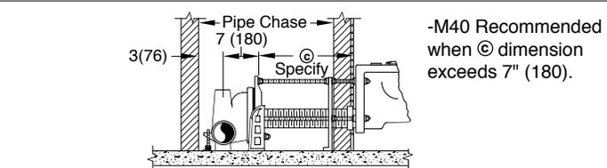
Illustration shows single installation. For double (back to back) installations specify whether -M40 variation is required on one side or both sides of pipe chase. When ordering, the pipe chase width and Ⓢ dimension should also be specified.
