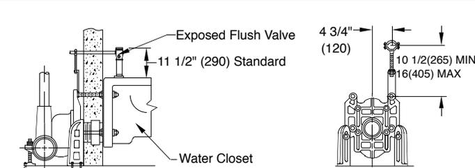
Provides support and alignment for the supply pipe to an exposed flush valve; must be specified for either 1" (25) copper tube or 1" (25) iron pipe.
