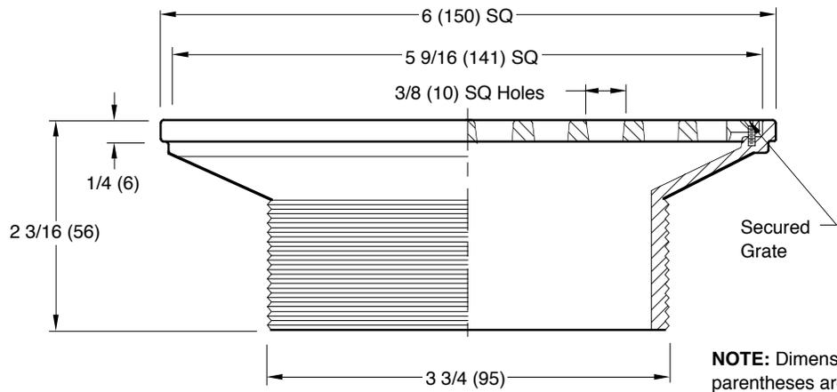
**NOTE:** Dimensions shown in parentheses are in millimeters.
