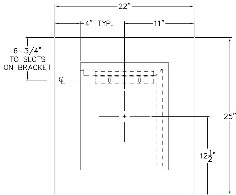
NOTE: NEO-METRO RECOMMENDS THAT WALL STUD OR ADEQUATE WALL BACKING BE UTILIZED OR PROVIDED FOR WALL-HUNG INSTALLATIONS. WALL ANCHORS AND ANCHORING FASTENERS ARE PROVIDED BY OTHERS.
