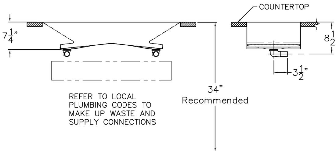
REFER TO LOCAL PLUMBING CODES TO MAKE UP WASTE AND SUPPLY CONNECTIONS
