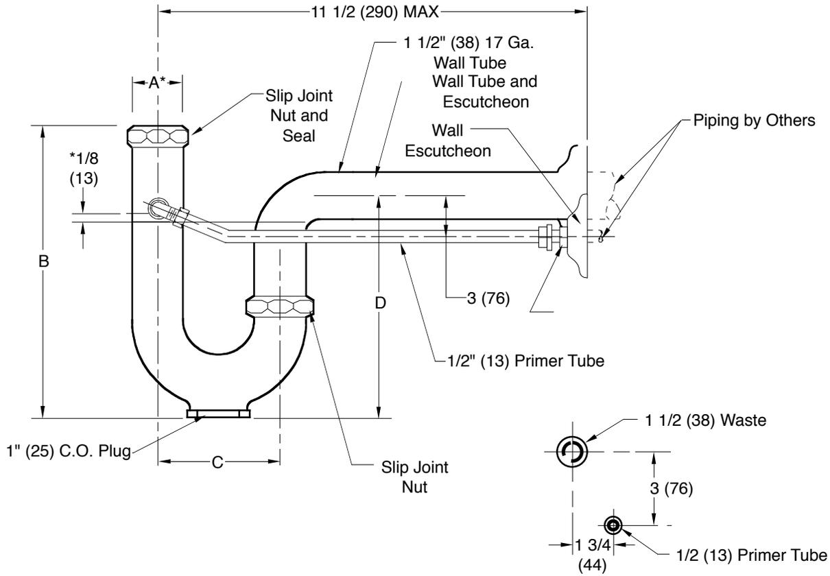
\*1 1/4 (32) and 1 1/2 (38) Slip Joint Nuts are Provided to Accommodate the Appropriate Fixture Tail piece. Ground Joint Elbow is Threaded 1 1/2 (38) N.P.T.
