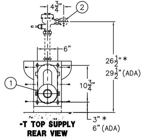
**NOTE: USE ONLY APPROPRIATE UPC/cUPC CERTIFIED FLUSH VALVE FOR THE INSTALLATION OF THIS TOILET.**
