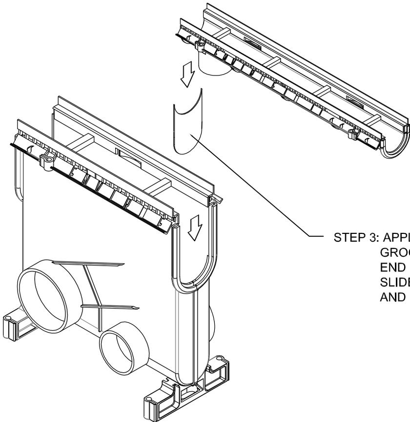
STEP 3: APPLY CHEMCALK 900 SEALANT INTO GROOVE IN CATCH BASIN. SLIDE SHALLOW END CAP INTO CATCH BASIN SLOT, THEN SLIDE TRENCH CHANNEL ON TOP OF END CAP AND SEAL WITH CHEMCALK 900 SEALANT
