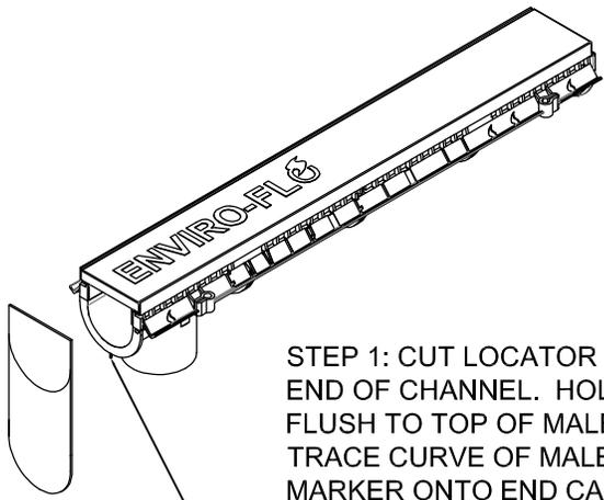
STEP 1: CUT LOCATOR PIN OFF BOTTOM OF MALE END OF CHANNEL. HOLD SHALLOW END CAP FLUSH TO TOP OF MALE END OF CHANNEL. TRACE CURVE OF MALE END OF CHANNEL WITH MARKER ONTO END CAP.
