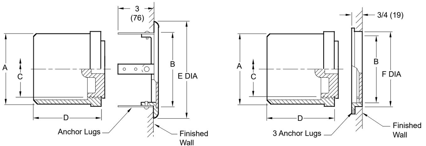
FIG. 4436C . . . . FACE-OF-WALL COVER
