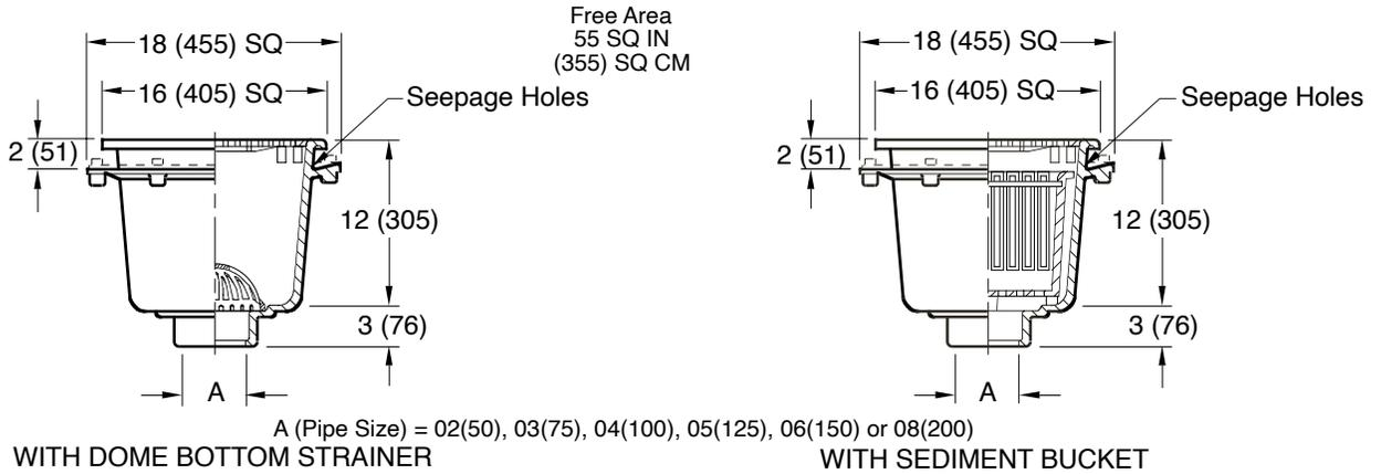
Fig. 3450C ... CAULK OUTLET ... Fig. 3451C
