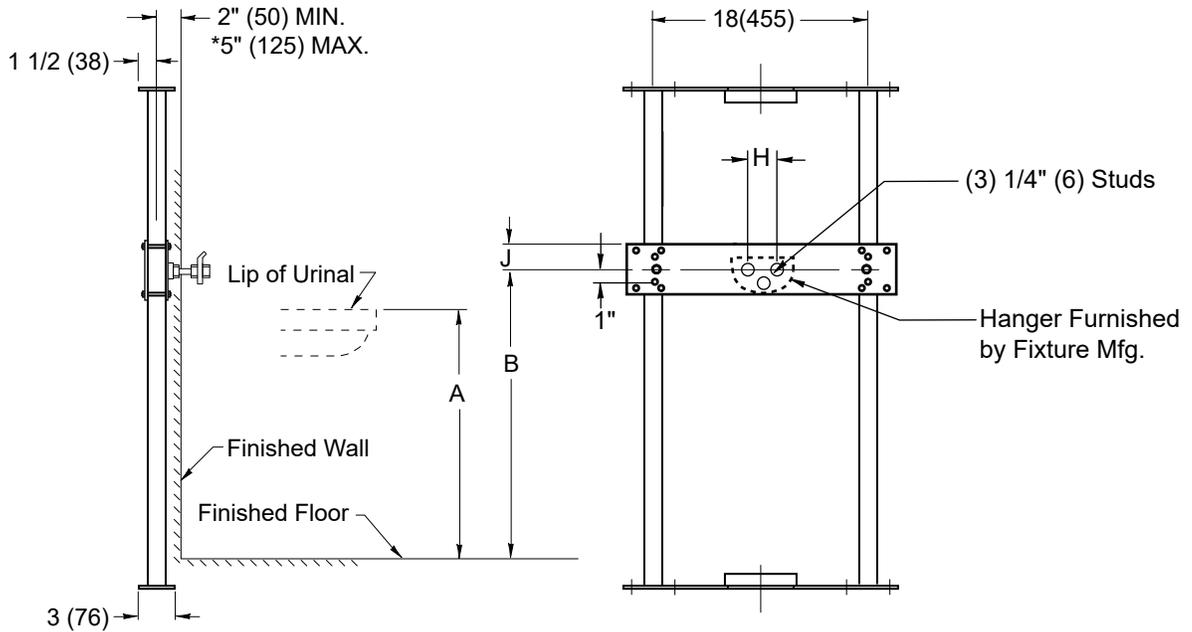
**NOTE:** The rough-in dimensions listed on this drawing are based on current information available to Jay R. Smith by the fixture manufacturers. We recommend that you verify these dimensions with the fixture manufacturer. We will not accept responsibility for rough-in dimension changes by the fixture manufacturer.
