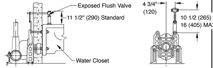
Provides support and alignment for the supply pipe to an exposed flush valve; must be specified for either 1" (25) copper tube or 1" (25) iron pipe.
