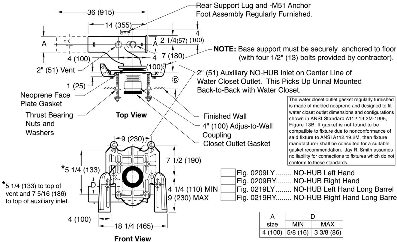
The water closet outlet gasket regularly furnished is made of molded neoprene and designed to fit water closet outlet dimensions and configurations shown in ANSI Standard A112.19.2M-1995, Figure 13B. If gasket is not found to be compatible to fixture due to nonconformance of said fixture to ANSI A112.19.2M, then fixture manufacturer shall be consulted for a suitable gasket recommendation. Jay R. Smith assumes no liability for connections to fixtures which do not conform to these standards.
