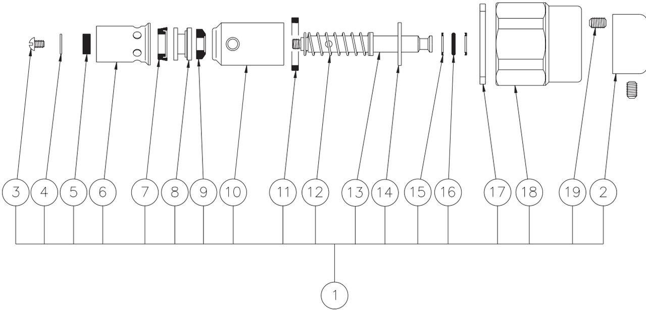
A-TIMING IS ADJUSTABLE FROM 5 TO 30 SECONDS. TURN THE SCREW, ITEM #3, CLOCKWISE TO INCREASE TIMING COUNTERCLOCKWISE TO DECREASE TIMING. CHANGES IN WATER TEMPERATURE WILL AFFECT TIMING AND MAY REQUIRE READJUSTMENT.
