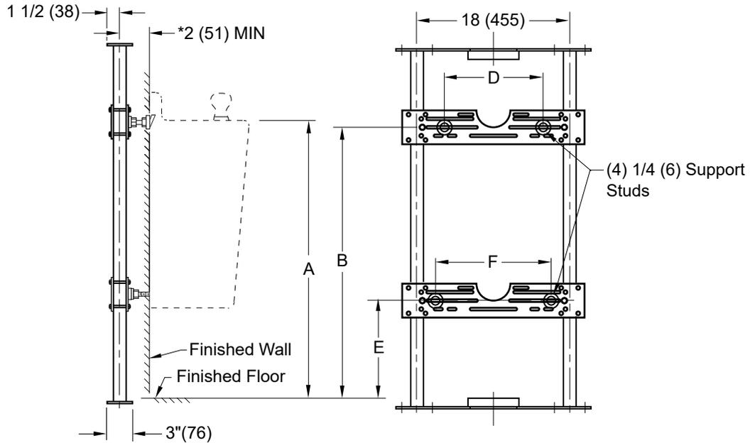
**Fig. 0831. . . FOR WALL MOUNTED ELECTRIC WATER COOLERS**
