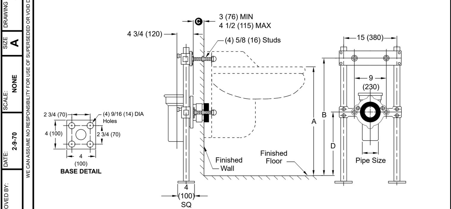
**Fig. 0915 . . . WITH SUPPORTING STUDS, ADJUSTABLE COUPLING AND WASTE FITTING 4" (100) CAULK AND 4" (100) VENT FOR BACK OUTLET FLUSHING RIM SERVICE SINK**
