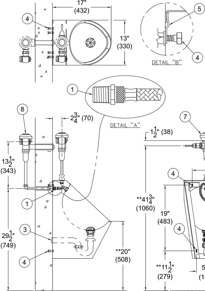
**NOTE: REFER TO ADA GUIDELINES FOR COMPLETE INSTALLATION REQUIREMENTS. ALL VERTICAL DIMENSIONS INDICATED (\*\*)
