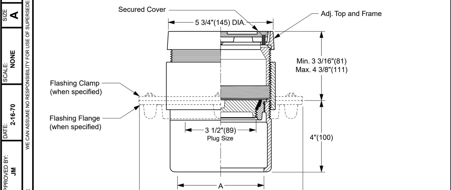
**NOTE:** For applications using core drilling, the largest diameter of the cleanout assembly is 6 5/16" (160).
