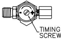
TIMING IS ADJUSTABLE FROM 5 TO 60 SECONDS AND IS ACCOMPLISHED BY ROTATING TIMING SCREW. TURNING THE SCREW CLOCKWISE INCREASES WHILE COUNTERCLOCKWISE DECREASES TIMING.
